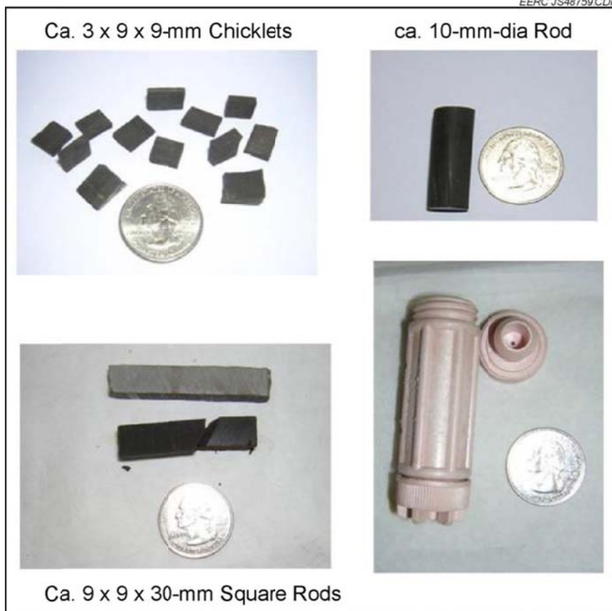
Figure 39. Typical reservoir and source rock samples prepared for CO 2 exposure. Samples are placed in the 10-mL extraction vessel (15 mm i.d. × 57 mm long, lower right), and exposed to CO 2 as described in the text.
