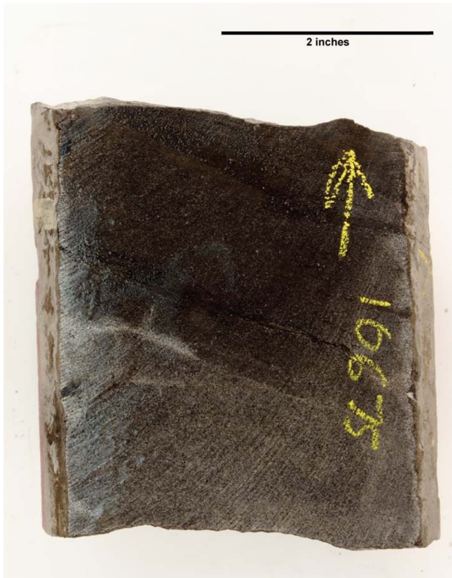
Depth 10675.2': A coarser, massive packstone. Open and cemented fractures are observed.
