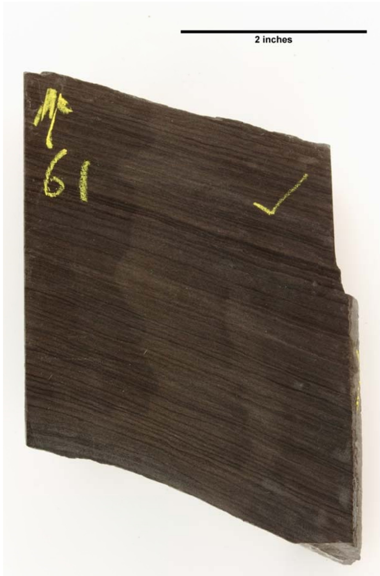
Depth 10561.1': A thinly rhythmic laminated siltstone. Bedding is angled.
