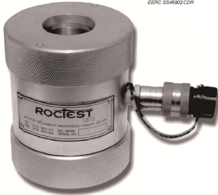
Figure B-2. Hoek cell used for applying confining pressure for triaxial testing.
