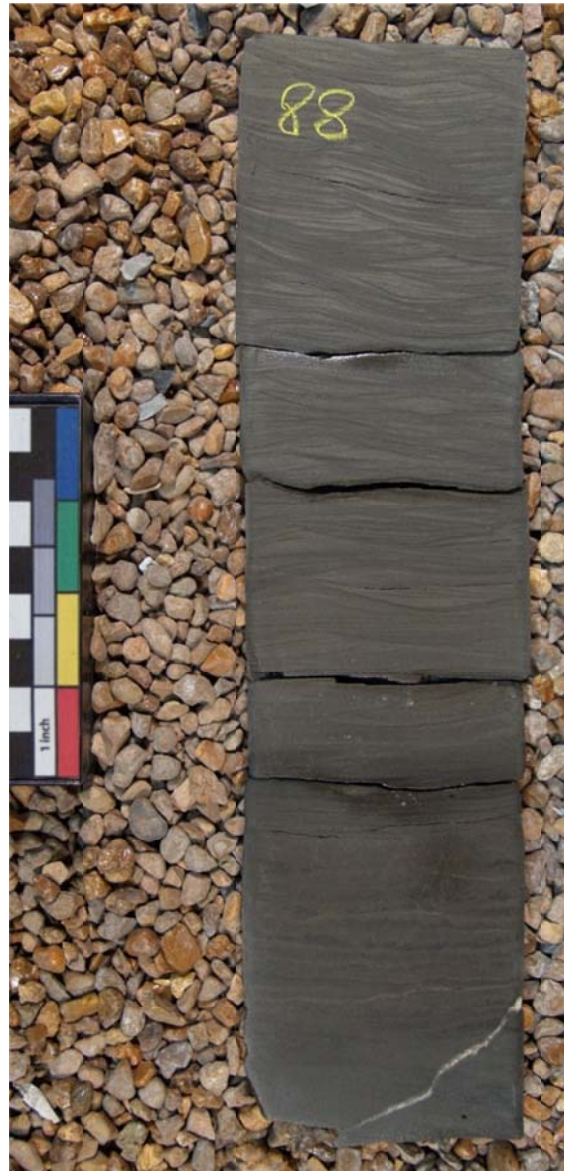
Depth 10688.5': A wispy laminated and cross-bedded siltstone.
