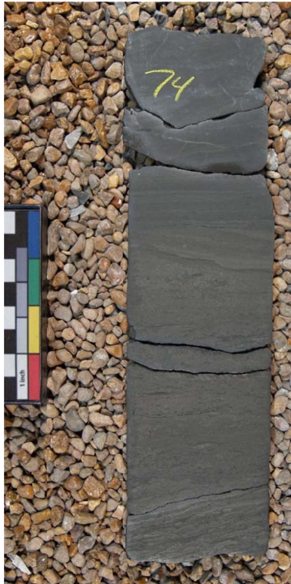
Depth 10674.0': Massive, dense, and fractured silty limestone.
