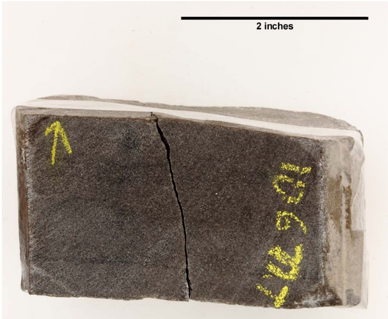
Depth 10677.8': A coarser, massive packstone. Open and cemented fractures are observed.
