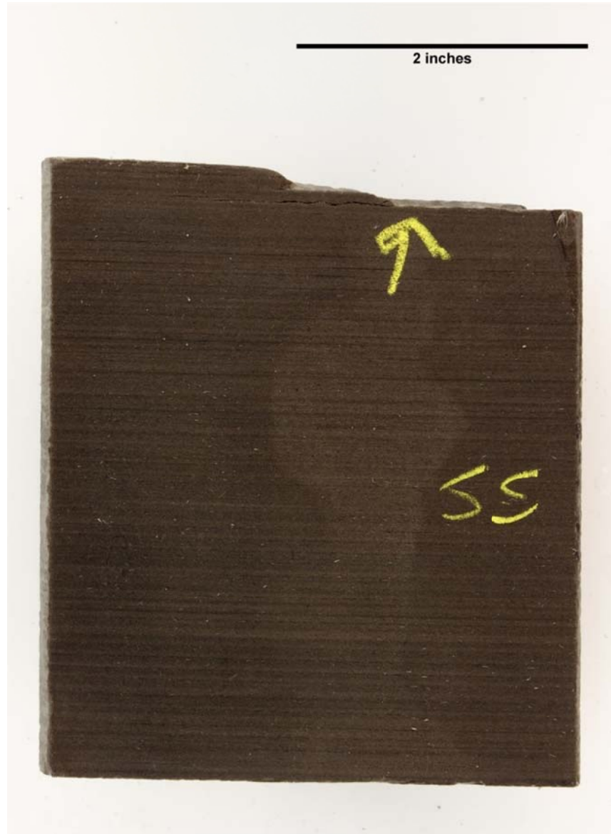
Depth 10555.0': A thinly paralleled laminated siltstone, perhaps a rhythmite feature.
