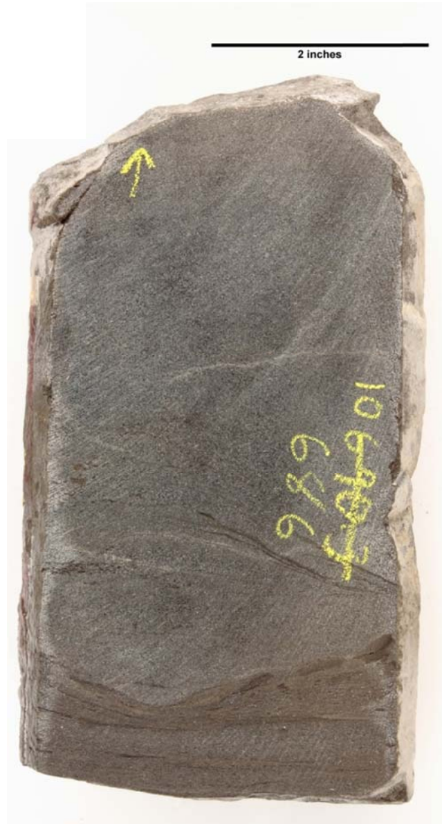
Depth 10686.0': A coarser, massive packstone. Cemented fractures are observed.
